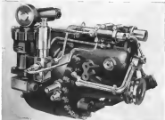
FRAZER-HAMILTON MANUFACTURED shafted product. Input shaft is at lower right, alternator mounts on the left.
